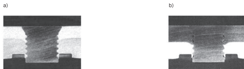
Fig. 5. Joint combinations: 2 aluminum sheets and steel/aluminum sheet: a) EN AW-6181A (g1 = 1.5 mm)/EN AW-5754 (g2 = 2.5 mm), b) EN 10130 (2.0 mm)/EN AW-5754 (g2 = 2.0 mm).
