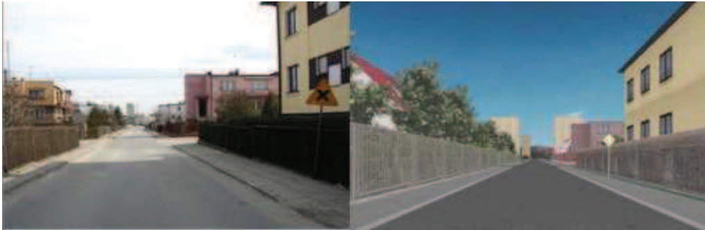
Fig. 2. The view on real road crossing and his mapping in AutoPW simulator.
