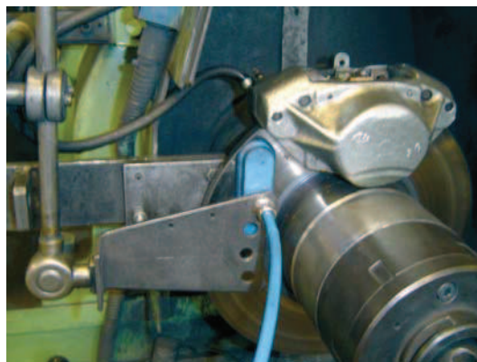
Fig. 4. View of the brake mechanism test setup and the location of the suction pad.
