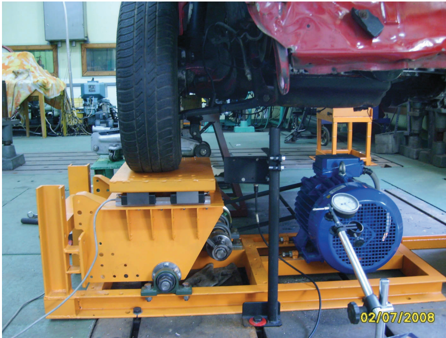
Fig. 2. The vibratory platform of the test stand
