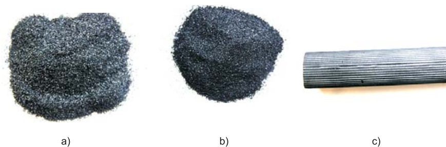
Figure 2. The example fuel samples: a) biocarbon, b) hard coal, c) graphite rod (d=13 mm).
