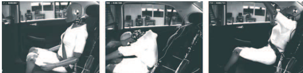
Fig.6. F5 dummy displacement on the P3 seat during frontal collision of a car with a rigid flat barrier at the speed of 56 km/h [8].
