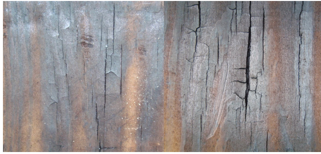
Fig 7. Views of non-treated pine timber specimen after tests with heat source of 8 kW/m 2
