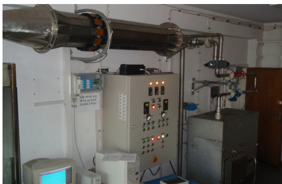
Fig 1. A view of the research equipment for the measurement of the concentration of toxic combustions products
