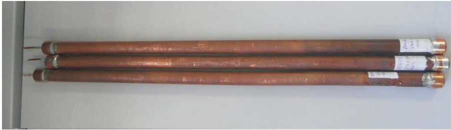
Figure 2. Water heat pipes with sintered capillary structure.
