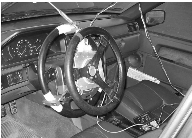
Fig. 2. Equipment used for measurements of steering wheel angle and steering torque.
