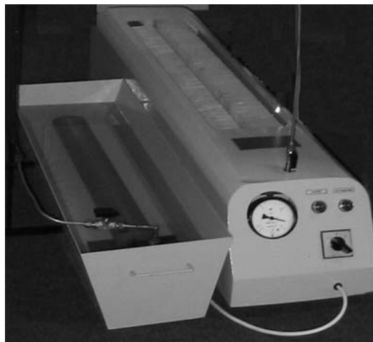
Figure 8. Two-adsorbers heat pump experimental set-up with evaporator for liquid cooling with COP = 1.6 .
