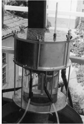
Figure 21. Reverse thermosiphon model integrated with a solar installation.
