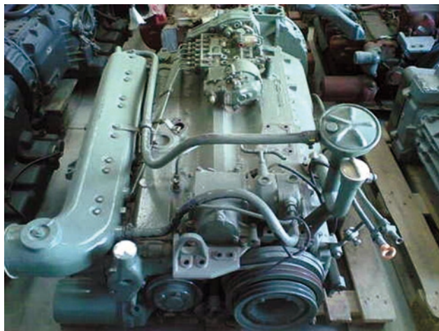
Podpodtłogowy, R6; V_{ss} = 11,967 \text{ dm}^3 ; D = 128 \text{ mm} ; S = 155 \text{ mm} , N_e = 147 \text{ kW}/2200 \text{ obr./min} ; M_o = 716 \text{ Nm}/1400 \text{ obr./min} ; g_e = 232 \text{ g/(kWh)}
