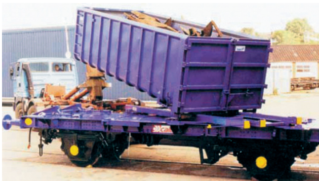
Fot. 10. Wagon RORA (Rail to Road) ACTS operatora CAIB UK [16]
