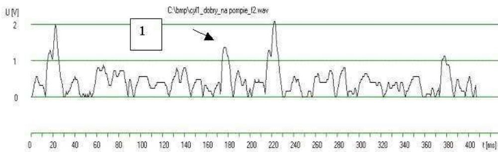
Fig. 7. Acoustic signal registered on the stub outlet of the pump feeding the injector working correctly. Mark „1” denotes a pulse to compare with a missing one shown in Fig. 10
