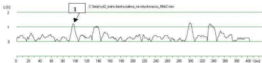
Fig. 9. Acoustic signal registered on the stub inlet to the injector in the situation when the fuel pump is out of trim and delivers less fuel into injector. The signal amplitude is smaller than that shown in Fig. 5.
