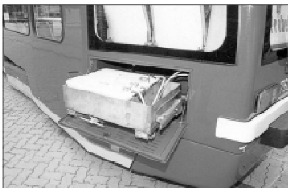
Fot. 8. Rostock – 4NBWE, akumulator Hoeppecke
