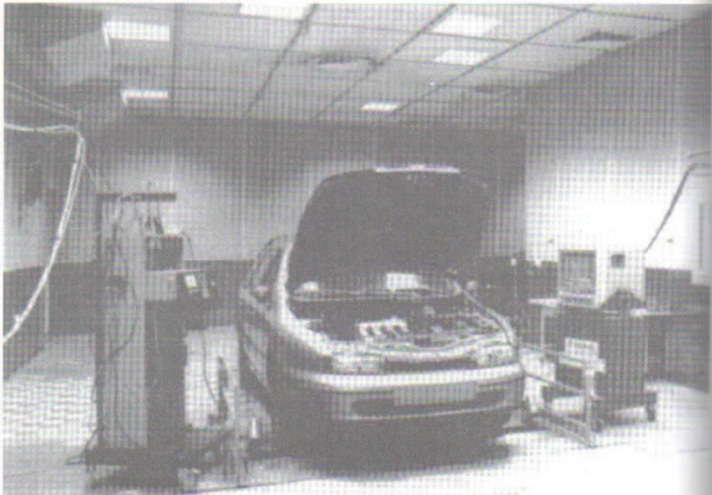
Fig. 8. View of the emission testing laboratory — testing cell with chassis dynamometer
