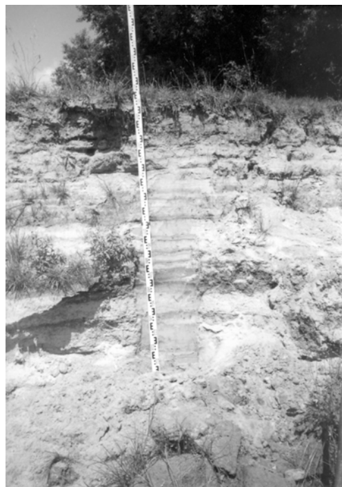
Phot 2. Soil layers on the channel slopes visible after erosion
