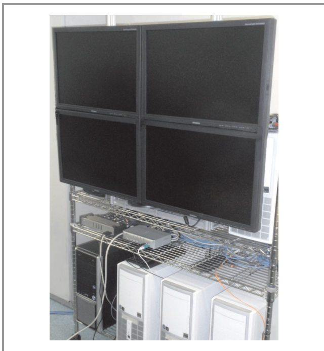
Fig. 2. Example of tiled display wall environment.
