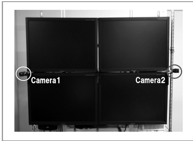
Fig. 4. Cameras setting on tiled display wall.
