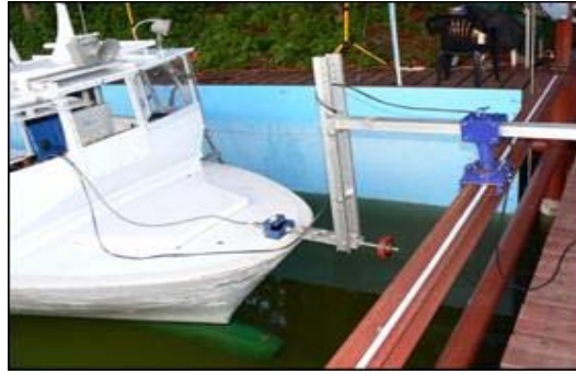
Fig. 1. Experimental test setup, bow pantograph
