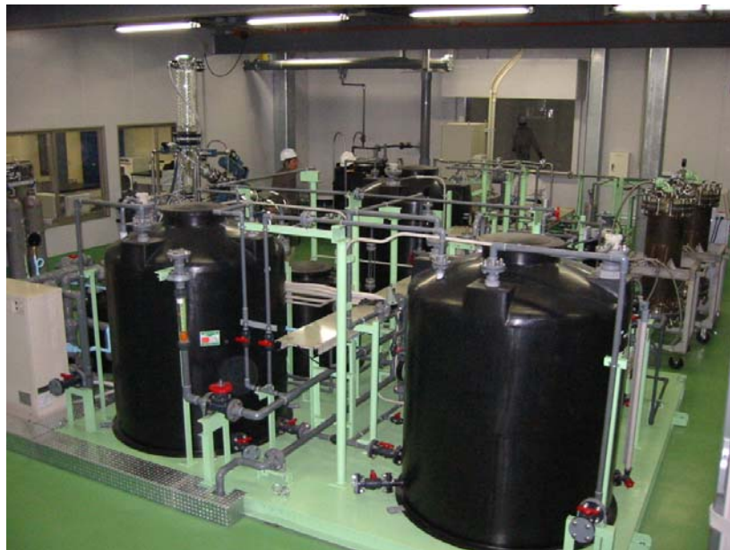
Fig. 3. Overview of the benchmark plant for selective lithium recovery.
