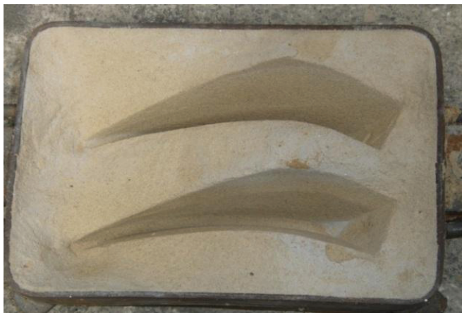
Fig. 9. Pattern match for the examined cast blades
