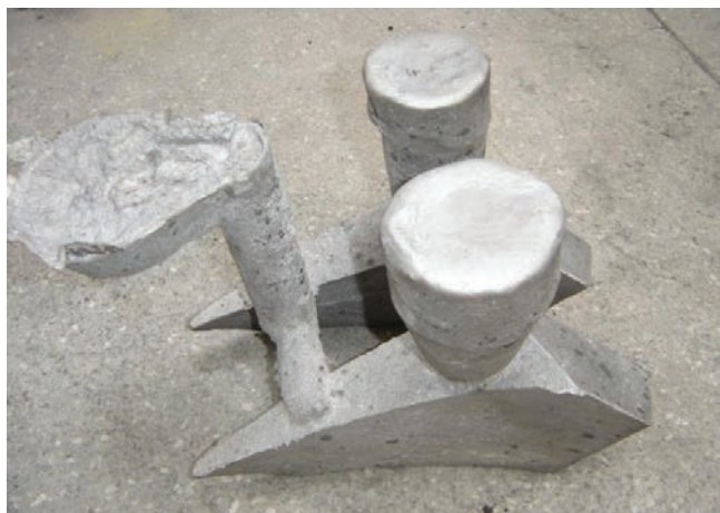
Fig. 12. Casting after fettling and removal of moulding sand
