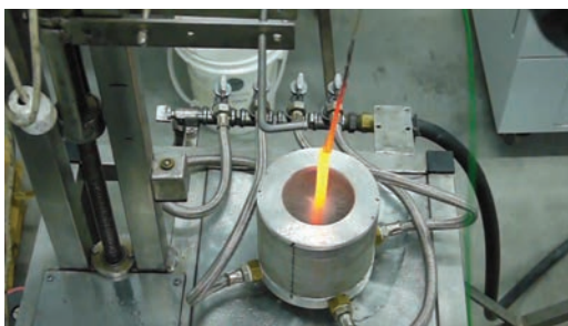
Fig. 3. The course of microjet solution heat treatment
