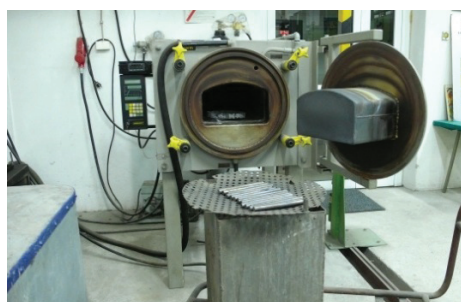
Fig. 4. General view of the heat treatment furnace with samples prepared for testing
