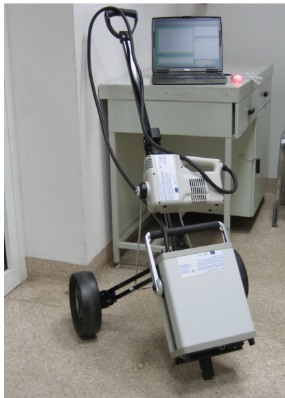
Rys. 2. zNose Model 4300 Ultra-Fast GC Analyzer
