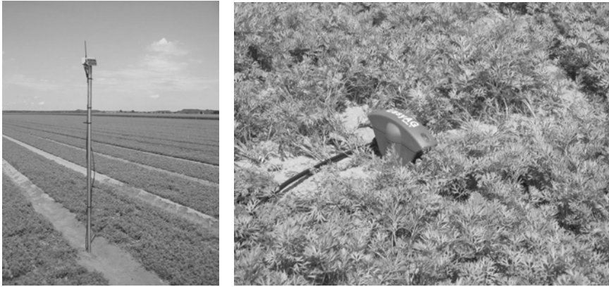
Fig. 4. Adcon transmitter and EasyAG probe on a field planted with baby carrots
