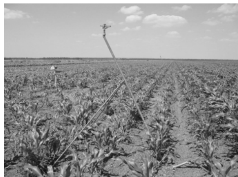
Fig. 3. EnviroSCAN (Sentek company) on fields planted with zucchini (left) and sweet maize (right)
