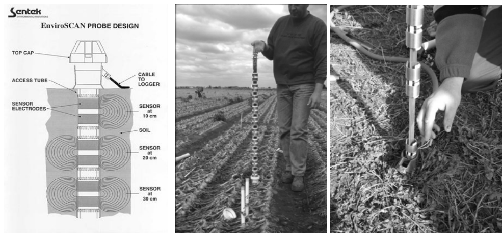
Fig. 5. Scheme of Sentek's EnviroSCAN with sensors and EasyAG (right)
