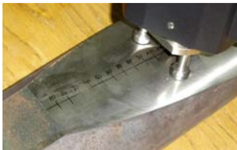
Fig. 1. Testing the effectiveness of heat treatment (austempering) by measurement of through-hardness in an austempered keel block
