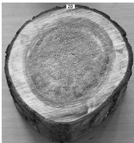
Fig. 1. Scots pine stem section with heartwood degraded by Phellinus pini (Thore) Fr.
