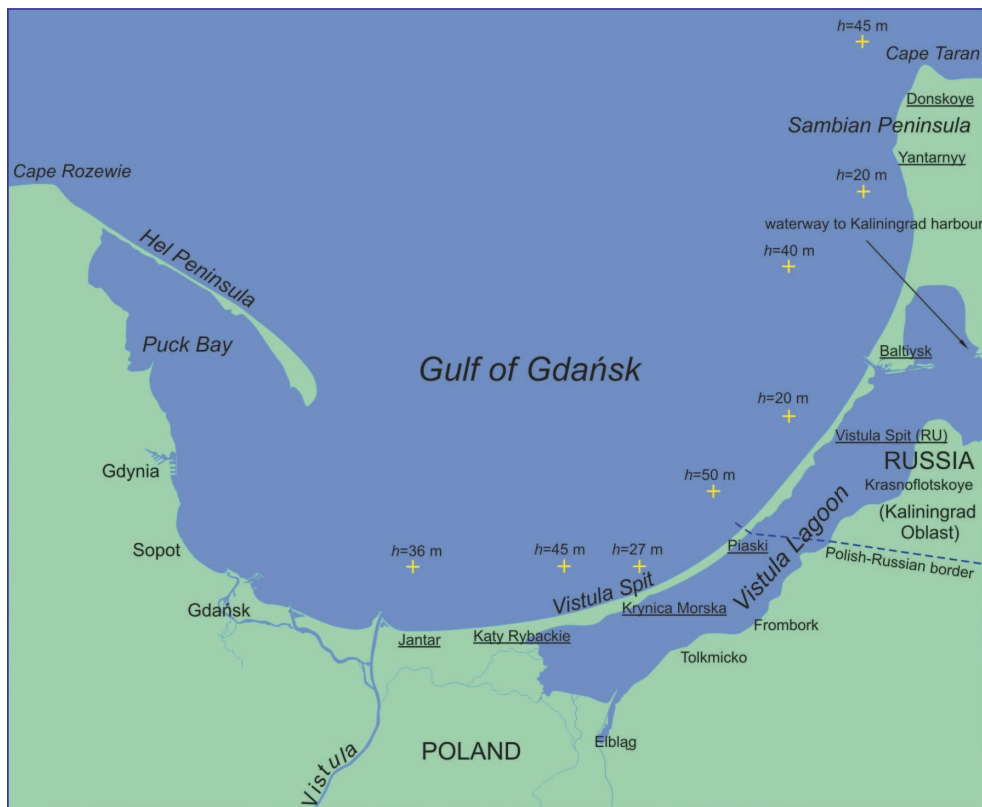
Fig. 1. Locations of deep-water wave prognostic points in the east part of the Gulf of Gdańsk
