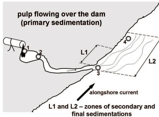
**Fig. 3.** Scheme of dumping of pulp (and sampling points 1–4) from a pipe line coming from the amber mining to the beach (A), grain size compositions (in %) for sampling points (B) shows the loss of coarse fractions while dumped waters are flowing over the dam (Determination ... 1994)
