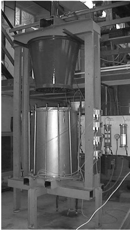
Fig. 2. View and cross-section of the calibration chamber at GUT (Bałachowski and Dembicki 2003)
