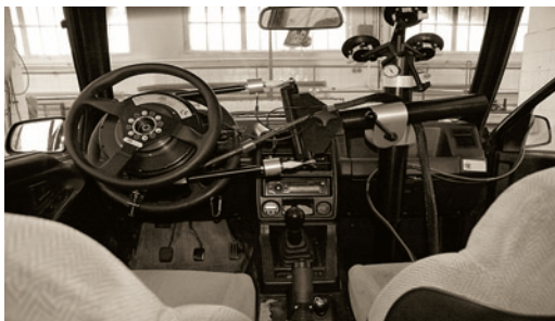
Fig. 1. A schematic of the instrumentation installed into the test vehicle and a cockpit view of the steering robot arrangement. 1, 2 – rotating wheel dynamometers, 3 – steering robot, 4 – interface computer; 5 – master computer; 6 – DGPS onboard unit, 7 – power supply
