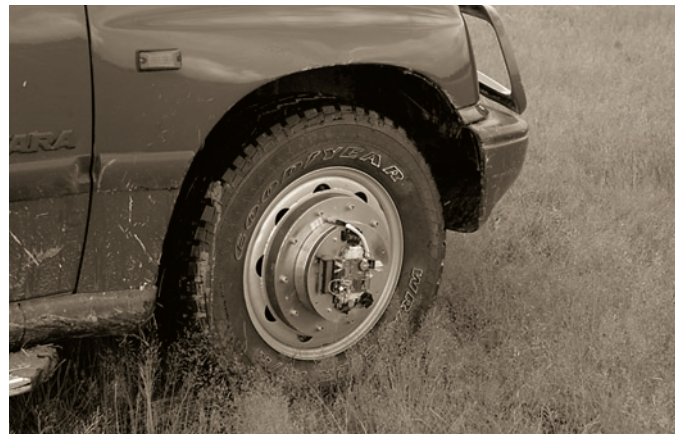
Fig. 1. A rotating wheel dynamometer installed on a test vehicle, during a test ride on a grassy surface. Braking moment M_y of a wheel is being measured
