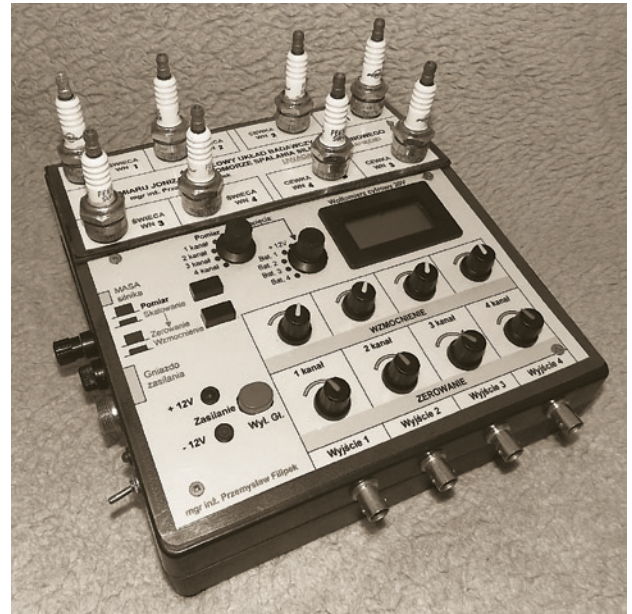
Fig. 3. Measuring system used to measure ionization current in four cylinders
