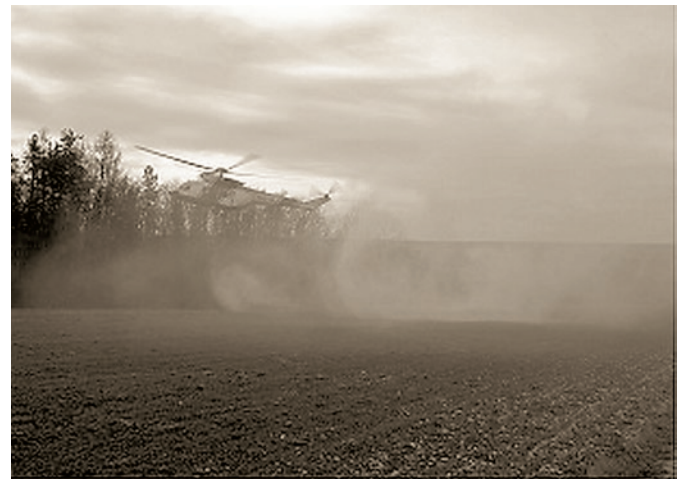
Fig. 10. The structure of the behind-rotor stream during experimental tests on the real helicopter W3-A FALCON
