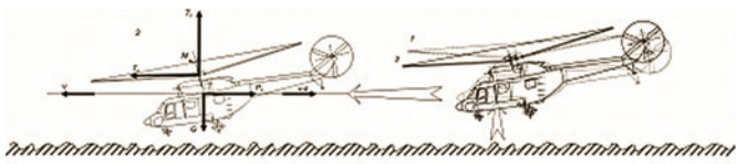
Fig. 11. Schematic diagram of the distribution of forces acting on the helicopter during the low hovering flight
