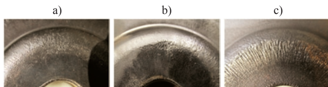
Fig. 2. Die insert wear after forging: a) 550, b) 1900 and c) 4300 pieces.
