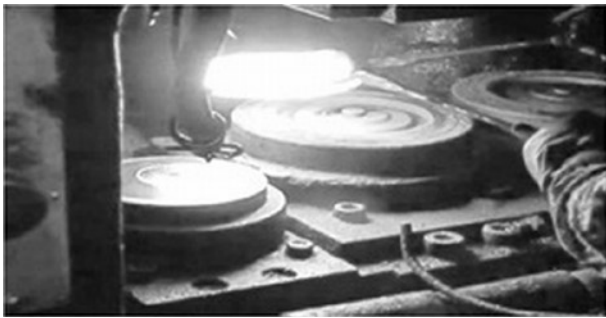
Fig. 1. Die inserts used in industrial hot forging.
