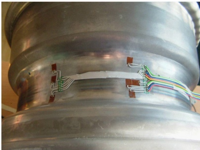
Fig. 2. The rim of the wheel with strain gauges in place from the tyre side
