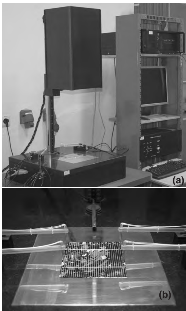
Fig. 1. Photos of I-V Curve Tracer For Solar Cells Qualification: a) general view, b) „table” with solar cells under four probes during measurement.
