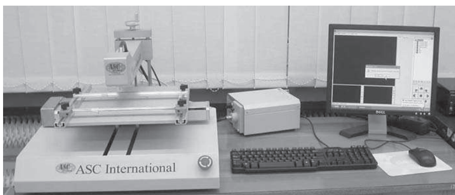
Fig. 2. 3D inspection system Vision Master AP.
