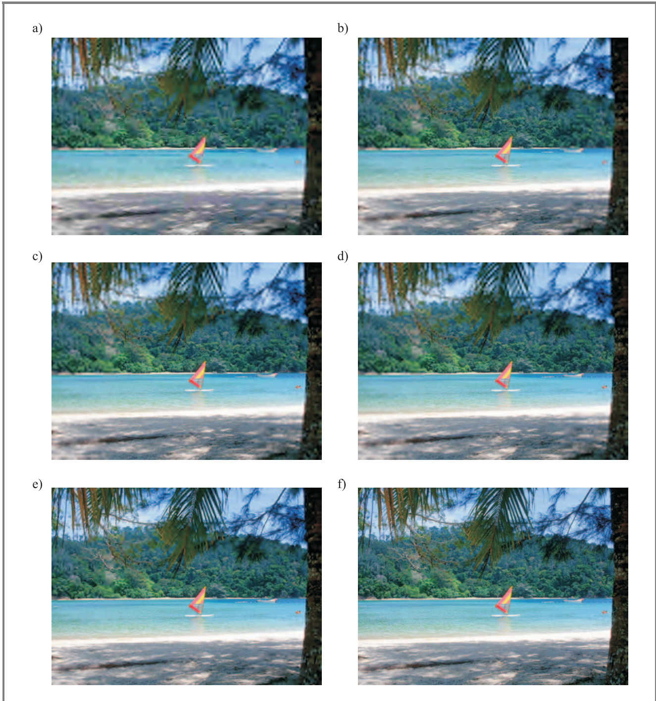
Fig. 5. Progressive decoding of a ROI prioritised code-stream at: (a) 0.0625; (b) 0.125; (c) 0.25; (d) 0.5; (e) 1.0; (f) 2.0 bits per pixel (bpp) for the beach image example in Fig. 4. The ROIs improve most rapidly at reduced bit-rates, while the visually lossless (or near-lossless) reconstruction of the image as a whole is possible at higher bit-rates.
