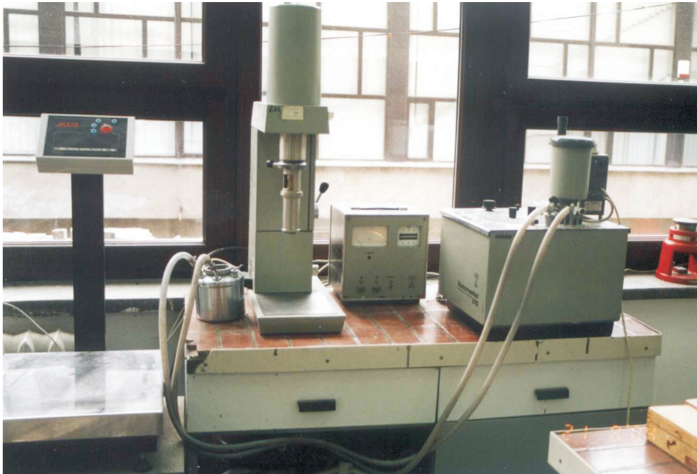
Fig. 1. The test stand for measurement of rheological properties of fresh gypsum pastes – RHEOTEST-2
