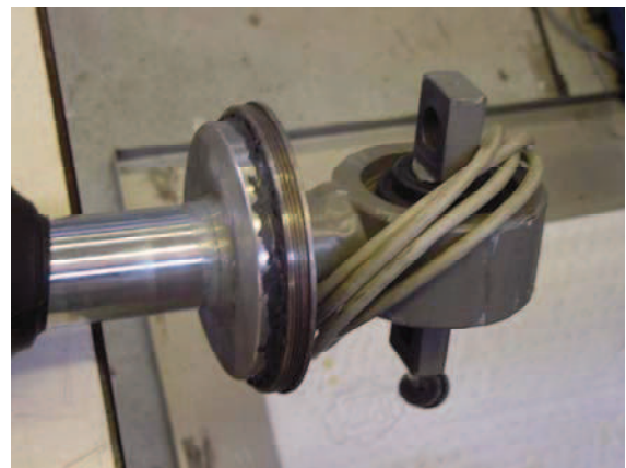
Figure 3: Strain gage attached to the piston rod (under metal shield)
