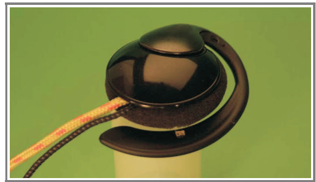
Fig. 6. Earphone-based sensor together with a recorder (© CSEM).
