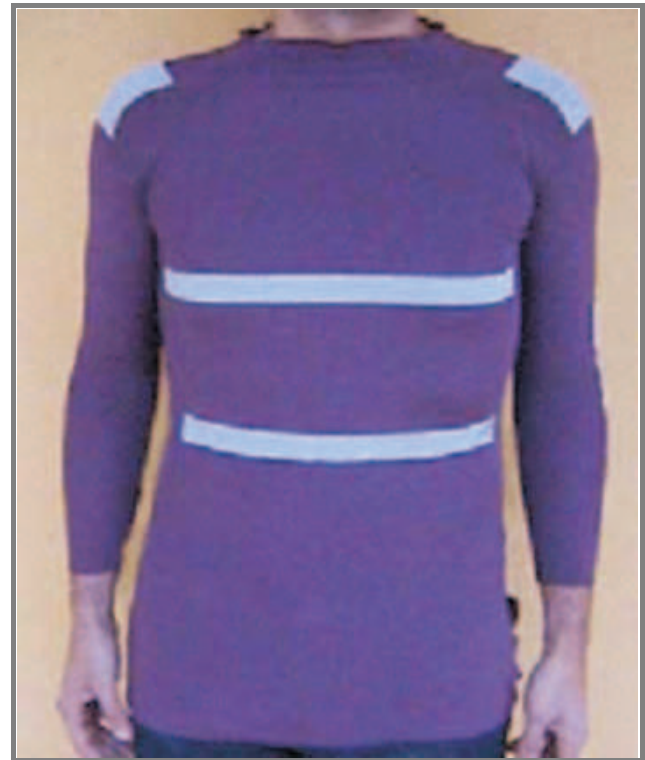
Fig. 3. Prototype of shirt with electrodes for movement measurement at shoulders and respiration bands (plethysmography) from the IST European project WEALTHY (wearable health care system).
