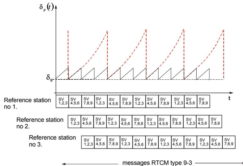
**Fig. 4.3.** A concept of multi-station system performance with telemetric link for chain of 3 DGPS reference stations and expected increase in the pseudorange accuracy measurement
