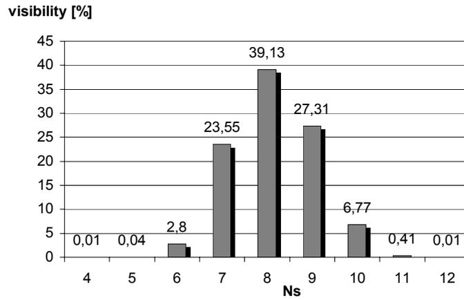
Fig. 3.6. The global GPS visibility (%). Total constellation of satellites - 24 SV [SPS, 1993]
