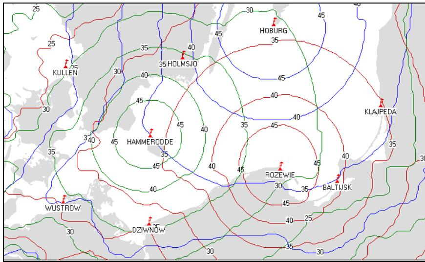
**Fig. 4.1.** Coverage areas of DGPS reference stations: Rozewie, Hoburg and Hammerodde
