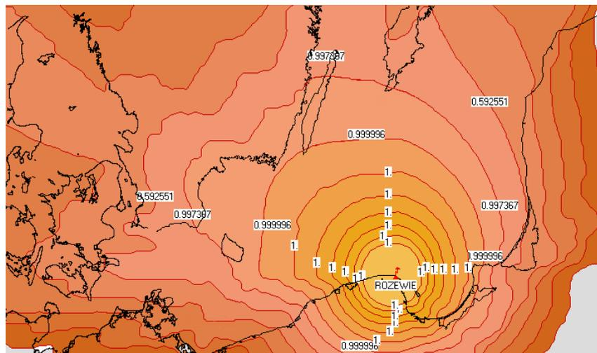
**Fig. 4.7.** Transmission availability of DGPS reference station Rozewie
