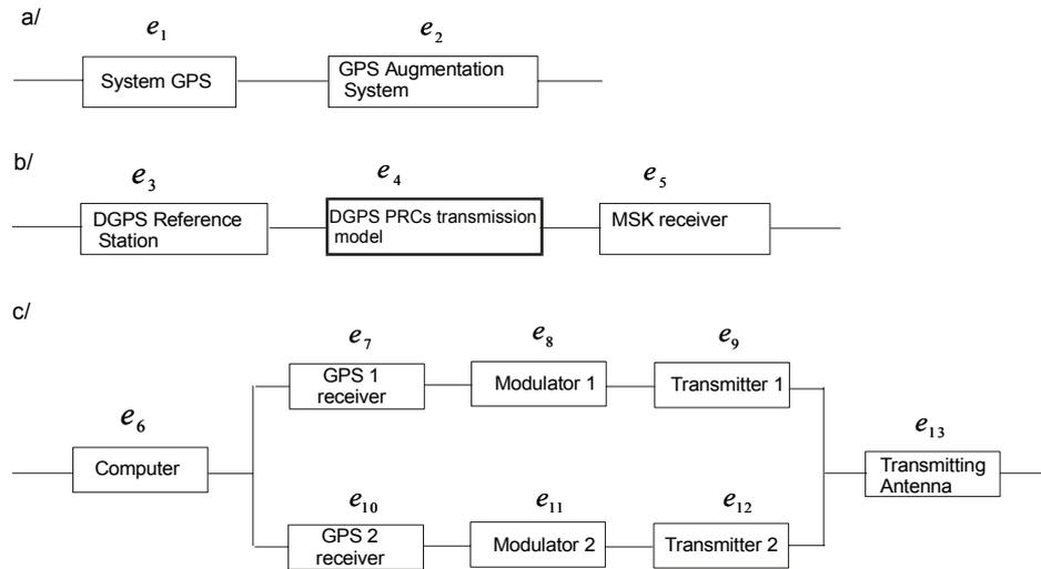
**Fig. 2.1.** The chosen navigational structures of the DGPS system: a/ the general structure of the system, b/ the structure of pseudorange corrections transmission, c/ the structure of the reference station
