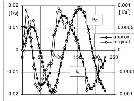
**Fig.5.** Calculated yaw velocity and acceleration
