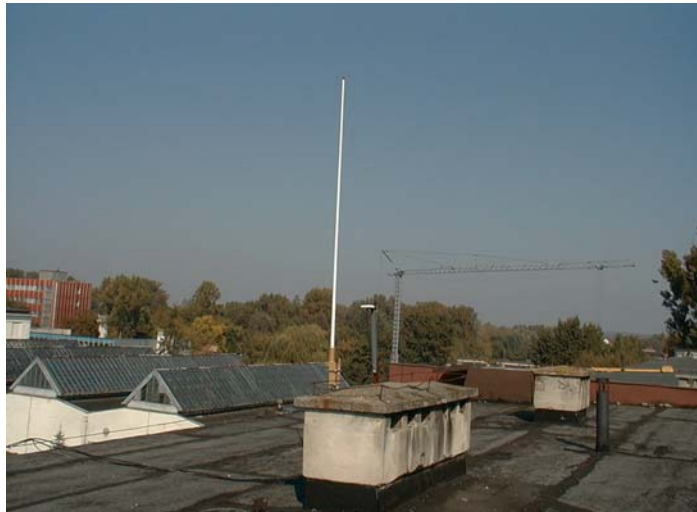
Photo. 1. CXL70-5C antenna of reference station
