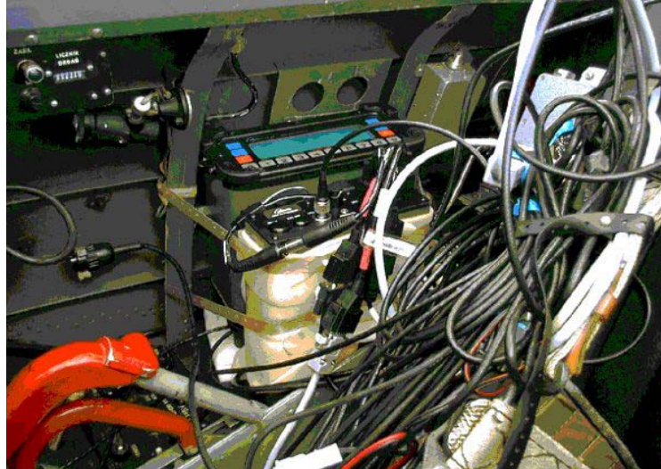
Photo. 3. The assembly of GG 24 and of Z12 receiver receivers in TS 11 cockpit
