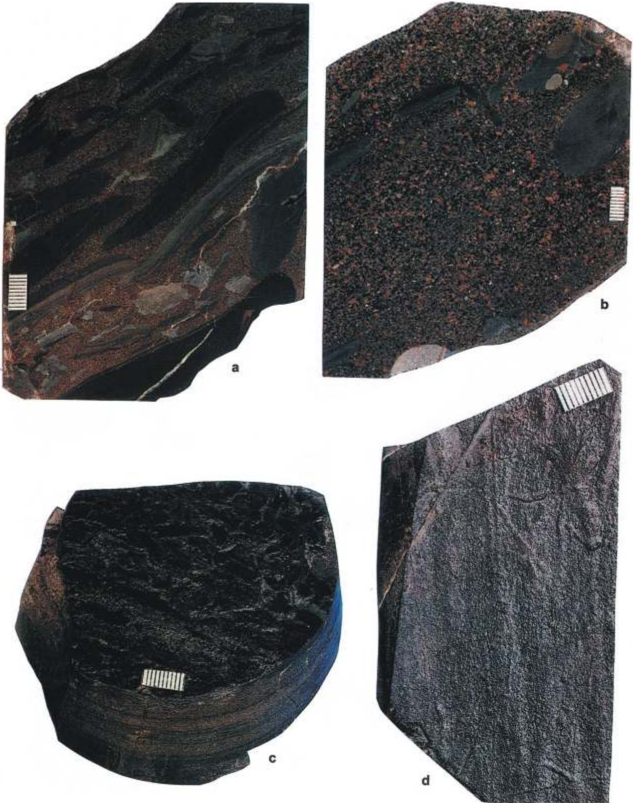
Fig. 6. a — facies 1; mud clast concentrations in fine-grained sandstone (wacke); elongate clasts are oriented parallel to the bedding; Ostałów PIG 2; depth 2562.7 m. b — facies 1; massive sandstone: medium- and coarse-grained wacke with mud clasts similar to those in Fig. 6a; in the top right, a fragment of mud-supported conglomerate is visible; Ostałów PIG 2; depth 2682.7 m. c — facies 2; horizontally laminated fine-grained sandstone; upper surface of one lamina with fragments of indeterminate coalified flora; the fragments are set parallel, indicating current origin of laminae; Ostałów PIG 2; depth 2644.3 m. d — facies 2; sole surface of horizontal lamina in fine-grained sandstone; small tool marks (bounce and groove marks) indicate current flow; Ostałów PIG 2; depth 2539.0 m
