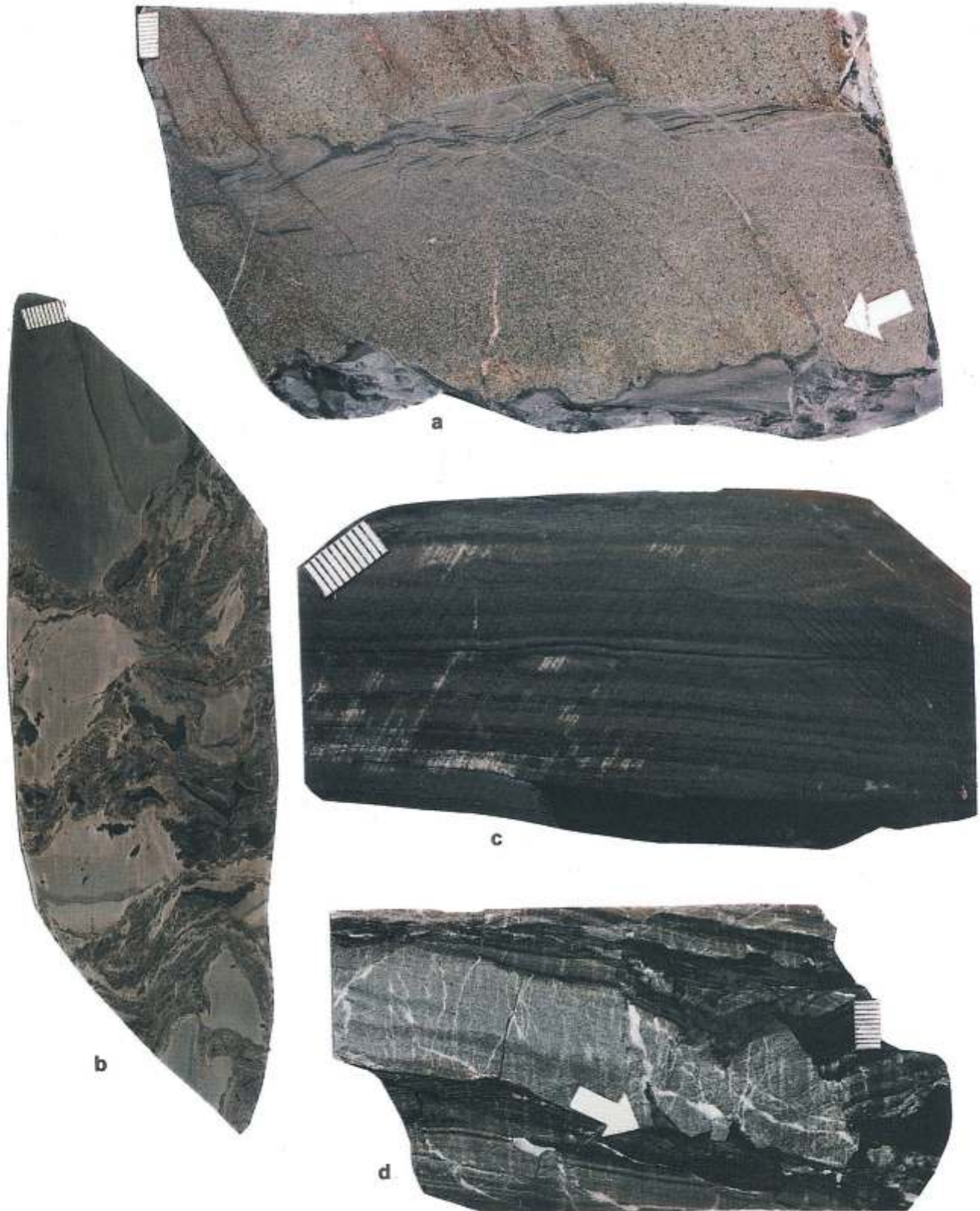
Fig. 7. a — facies 2; two thin beds of normally graded fine-grained sandstone; lower bed represents a Ta-c Bouma (1962) sequence truncated at the top; the distinct lower boundary of this bed is characterised by load casts; note sedimentary tension fractures caused by slow sliding of parallel-bedded deposits; one of the fractures is partly filled with upward-squeezed mud (arrowed); Opoczno FIG 2; depth 3004.5 m. b — facies 2; slump structure: randomly arranged fragments of broken and deformed siltstone and claystone beds in a sandy-clay matrix; Opoczno FIG 2; depth 2990.2 m. c — facies 3; sand/mud heterolith, subfacies 3A: sand-dominated heterolith; horizontal lamination, single sandstone lense and erosional scour filled with cross-laminated sandstone; Ostałów FIG 2; depth 2504.0 m. d — facies 3; sand/mud heterolith, subfacies 3B: mud-dominated heterolith; thin sandstone and siltstone beds with small-scale cross lamination; numerous tension fractures are visible; some fractures are filled with mud, squeezed out of mudstone interbeds; the arrowed fracture is filled with mud and calcite; Studzianna IG 2; depth 4045.0 m
