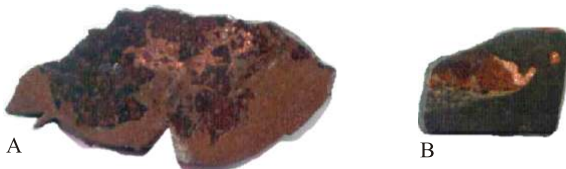
Fig. 10. A — knotty and veinlet-like concentrations of native copper in the basaltic volcanic breccia from the Policy quarry, natural size; B — fine grains of the native copper in goethite, sample SC 89.8 from borehole 5879, natural size
