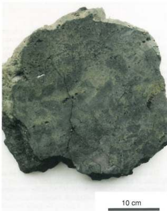
Fig. 2. On a cut surface the rock looks like a volcanic breccia with numerous brown-pink fragments immersed in the olive-black matrix
