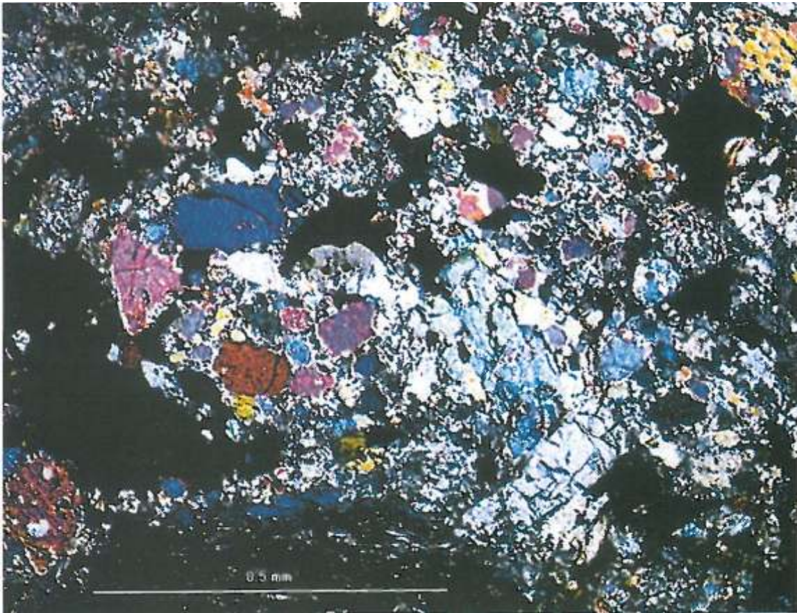
Fig. 9. Mt. Tazerzait; internally concise aggregate composed of chondrules, metal grains and olivine and pyroxene crystals (transmitted light, crossed nicols, x 100)
