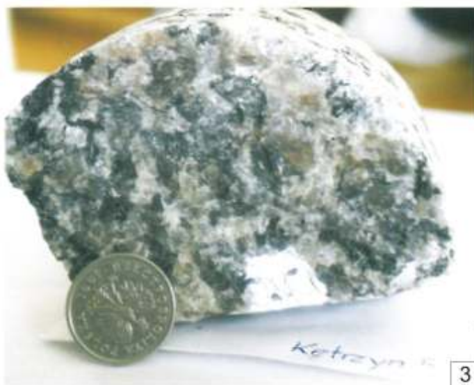
1. Porphyritic texture with large pink K-feldspar in charnockite from the Łanowicze drill-core; depth 1111.8 m. 2. Large plagioclase in quartz monzodiorite from the Filipów drill-core; depth 1553.0 m. 3. Porphyritic texture with large plagioclase crystals in quartz monzonite from the K. trzyn drill-core; depth 1549.5 m; diameter of the coin is 1.5 cm on all photos
