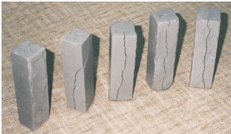
Photo 1. The samples of the slurry mixed with tap water (AW/R) after 69 days of storage in 1% solution of \text{Na}_2\text{SO}_4 , age of samples – 76 days
