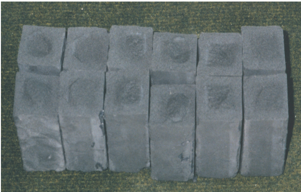
Photo 4. Fractures of slurry samples (BW/R) mixed with tap water and with the addition of ashes (after 90 days) stored for 76 days in 1% solution of \text{Na}_2\text{SO}_4
